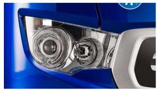
Compared with halogen headlamps, bi-xenon headlamps mean better illumination of the road
