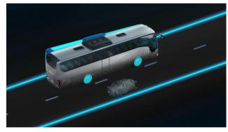
The Electronic Stability Program significantly reduces the risk of skidding by selectively braking individual wheels, thus preventing loss of control of the vehicle in curves and emergency steering manoeuvres.
